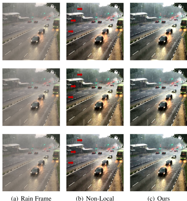
Fig. 13. Visual comparisons of the rain accumulation removal methods on two real rain sequences with heavy accumulation when the rain streak removal algorithm is not employed at the first stage. Our proposed non-local video rain accumulation method leads to more temporally continuous results than the single image-based method, especially in the regions denoted by red arrows. Zoom-in for better visualization.
